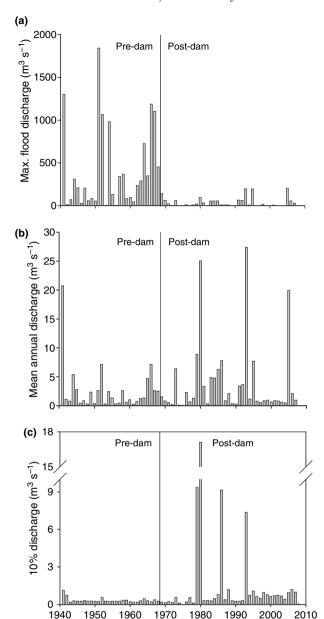
Fig. 2 Pre- and post-dam streamflow data for the Bill Williams River (1940-2007), as measured at the "Bill Williams River below Alamo Dam" stream gaging station. (a) Annual flood series; values are the largest peak instantaneous discharge in a given water year (Oct. 1 to Sept. 30). (b) Mean annual discharge. (c) 10% discharge (10% of flows are less than or equal to this in a given water year).
