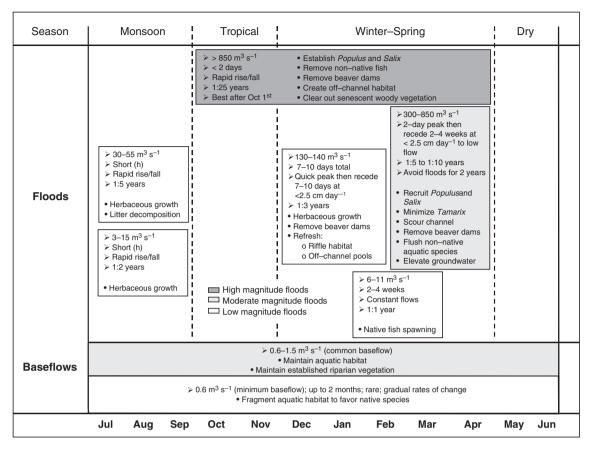
Fig. 4 Flow requirements for the Bill Williams River, developed by scientists and resource managers at a 2-day workshop. Blocks include different flood flow and baseflow regimes, within four seasons. Arrows indicate flow characteristics, such as magnitude, timing, duration, frequency and rate of change. Bullets indicate ecological functions associated with flows. See Shafroth & Beauchamp (2006) for more detailed information.
