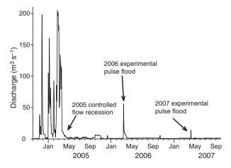
Fig. 5 Mean daily streamflow at the Bill Williams River near Alamo stream gage during a period with experimental flow releases from Alamo Dam and associated hydrology–ecology field research (from 1 Oct. 2004 to 30 Sept. 2007).
